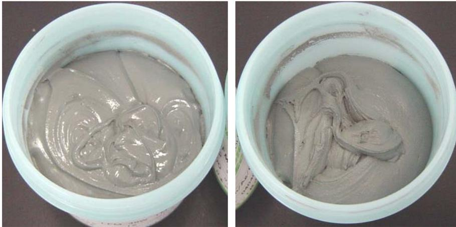
Paste in good condition / paste in poor condition
