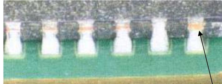
Exposed component termination = poor wetting.
