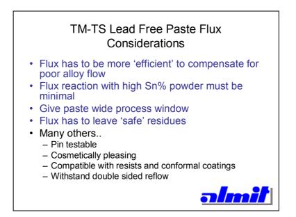
During the development of Almit TM-TS flux it was necessary to test it against the IPC standard for flux reliability and 'workabilty'. These standards are recognised as a minimum requirement for soldering fluxes that are to be used for high reliability applications. The summary of the tests performed for flux reliability and solder paste 'workability' are
